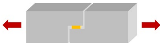
Figure 12: Thick adherend shear test
