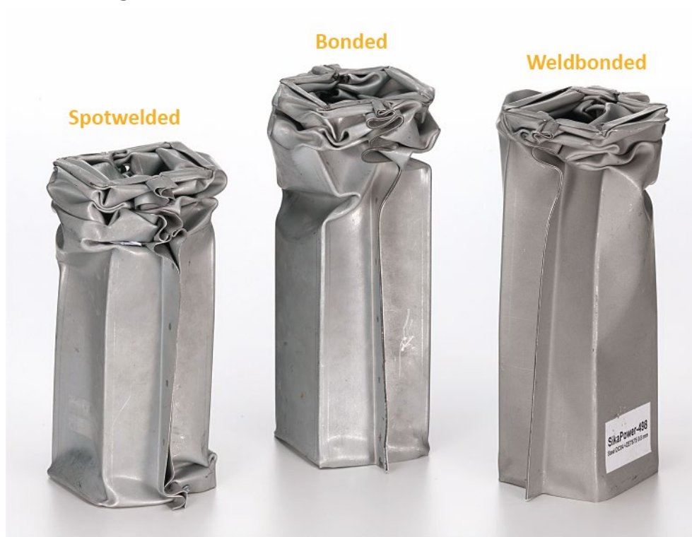
Figure 1: Spotwelded, bonded and weldbonded double hat profiles after crushing in a drop tower
