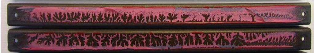
Figure 27: typical fracture surface showing viscous fingering
