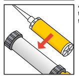
4. Place the cartridge into the gun and start application
