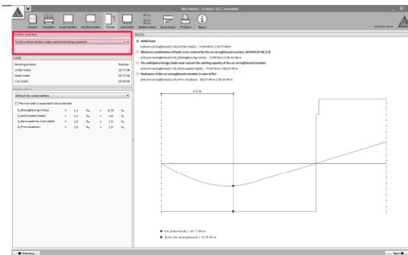
The calculation of the necessary FRP will be based on the critical section under positive or negative bending moments, as automatically determined by software.
