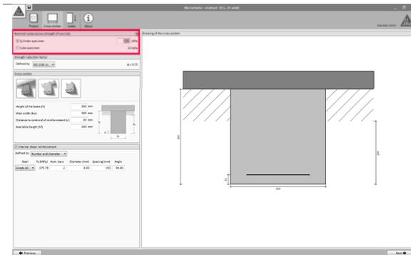
The compressive strength of the concrete ( $f'_c$ ) must be defined by the user.
