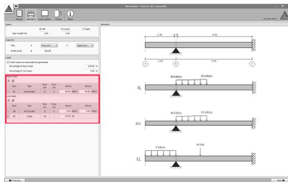
The arrangement of the un-factored dead and live loads along the element is done as follows:
