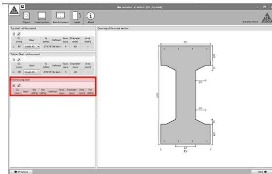
Additionally, bonded prestressing steel can be defined.
