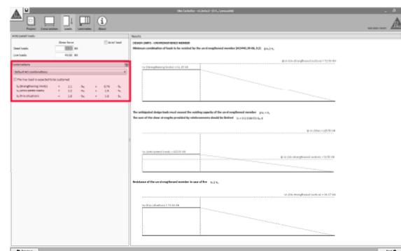
The different combinations of loads are indicated on the left side of the screen, showing the default combination factors as indicated in ACI 318 and ACI 440.2R-08.
