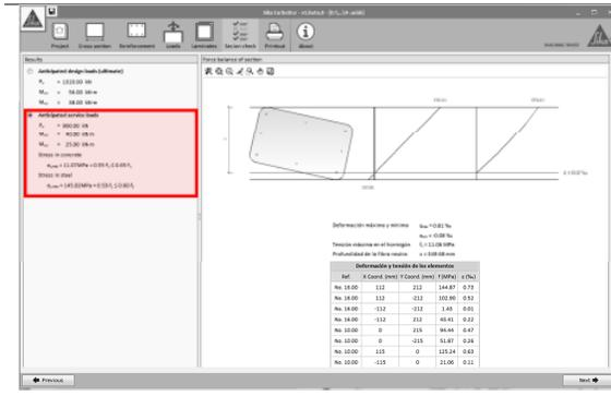
In the same way, the option corresponding to “anticipated service loads” shows the stress-strain profile of the strengthened section under the service loads.
