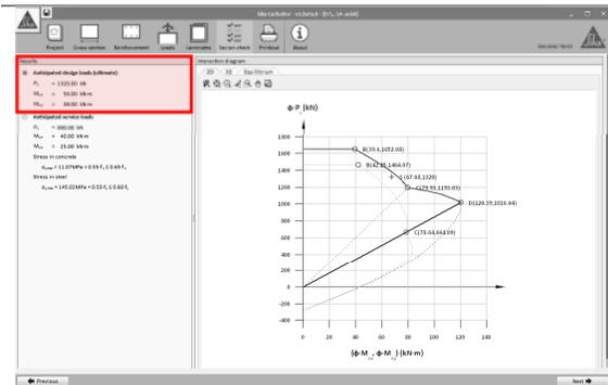
In the case that axial loads and bending moments act simultaneously (eccentricity larger than 0.1h), the information concerning the performance of the strengthened member under design loads will be substituted by an interaction diagram.
