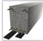
**Flexural strengthening of the critical section in a beam.**
