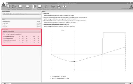
Different combinations of loads are indicated on the left side of the screen, showing the default combination factors as indicated in ACI 318 and ACI 440.2R-08.
