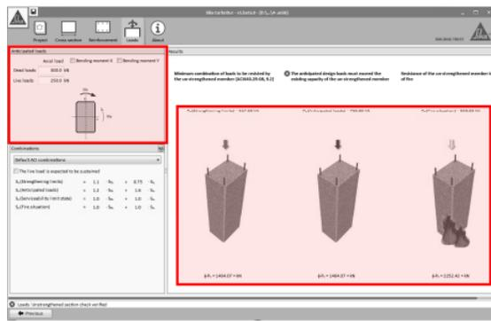
Pure axial loads are requested as default. Optionally, the user can activate the options corresponding to “Bending Moment X / Y”, which allow to enter additional bending moments acting in 1 or 2 different directions.
