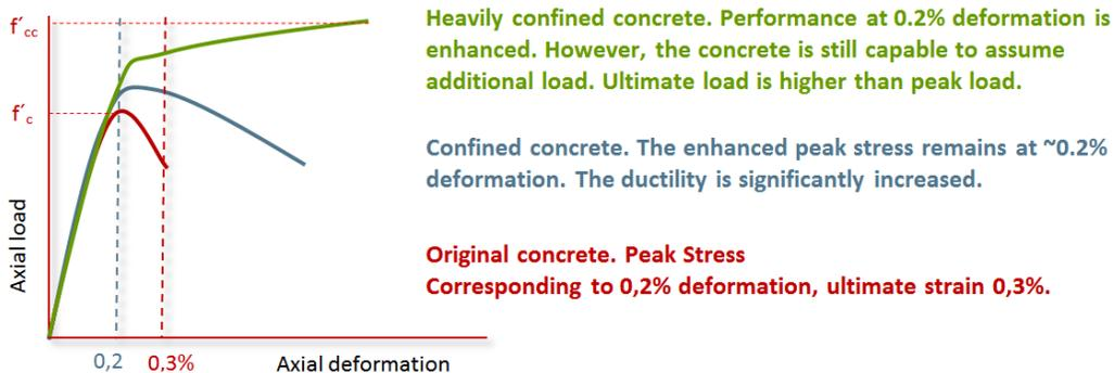
The figure displays a nearly bilinear response with a sharp softening and a transition zone at a stress level that is near the strength of unconfined concrete,  $f'_c$ . After this stress the tangent stiffness changes, until the concrete reaches its ultimate strength  $f'_{cc}$  when the jacket reaches tensile strain at failure  $\epsilon_{fe}$ .
