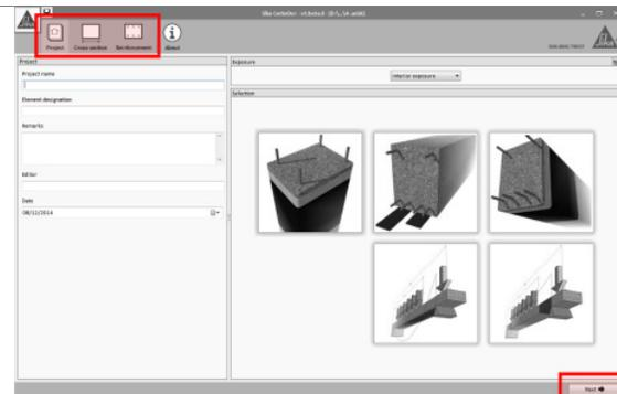
Regardless of the type of strengthening selected, the calculation process is organized into successive stages, which are shown in the icons situated at the top of the screen. The type and quantity of stages vary as a function of the selected strengthening method and the data introduced by the user.
