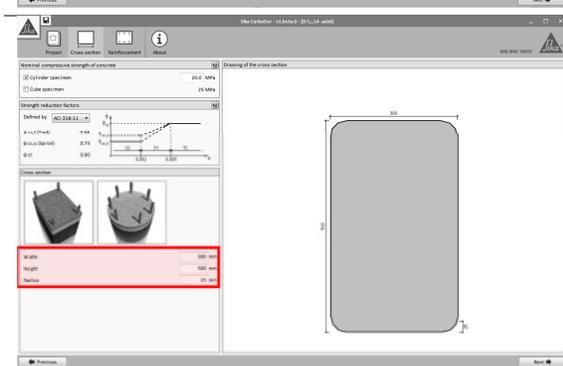
The dimensions of the cross section are entered in the boxes situated below the selection drawings.
