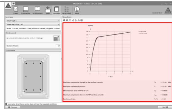
The main screen displays the stress-strain model corresponding to the un-confined and confined concrete. Axial strain is shown in the horizontal axis and the stress is displayed in the vertical axis.
