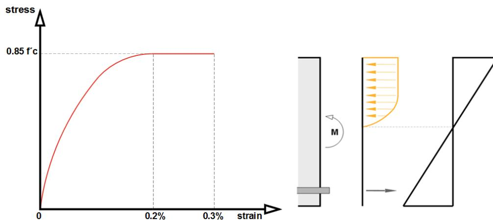
Concrete stress is determined according to the following equations:
