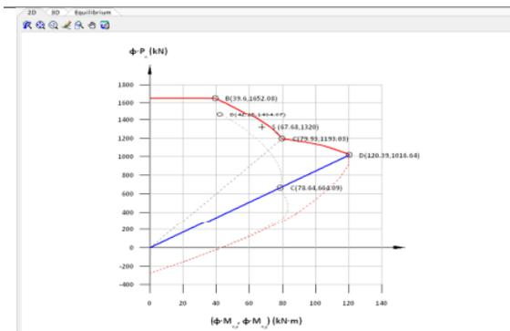
The 2D option shows simultaneously the ultimate strength of the un-strengthened (dashed) and strengthened (solid red) members, as well as the balance lines and the most relevant figures of the 2D profiles. The actual combination of design loads is shown in the same diagram as a cross symbol.
