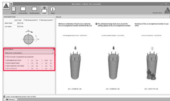
The different combinations of loads are indicated on the left hand side of the screen, showing the default combination factors as indicated in ACI 318 and ACI 440.2R-08.
