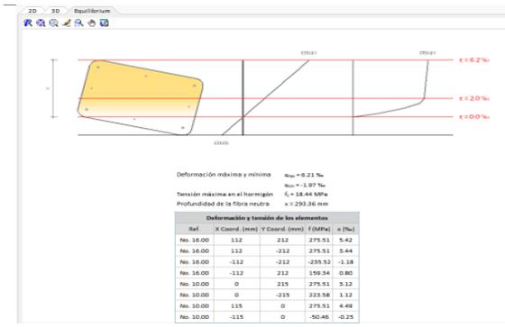
The tab named as “equilibrium” shows the stress-strain profile of the section under the combination of design loads.
