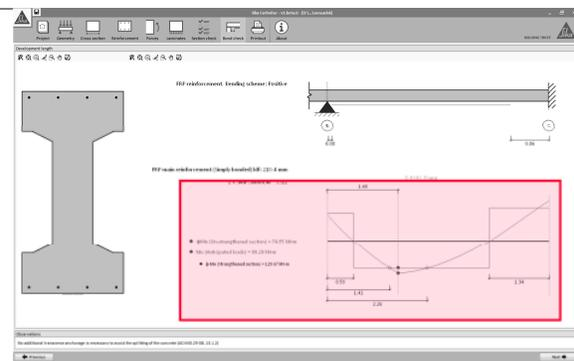
The bending diagram on the main screen displays the distribution of the bending moments corresponding to the anticipated design loads, as well as the original strength of the un-strengthened member.
