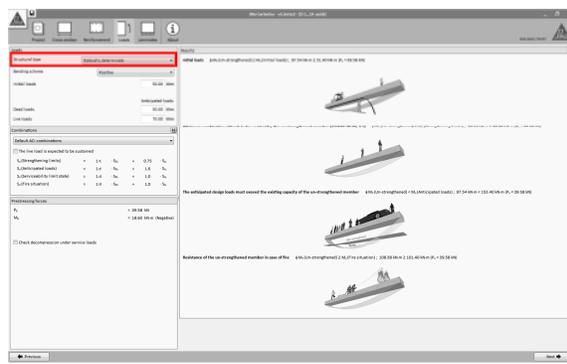
The user must indicate if the member is statically determinate or indeterminate.
