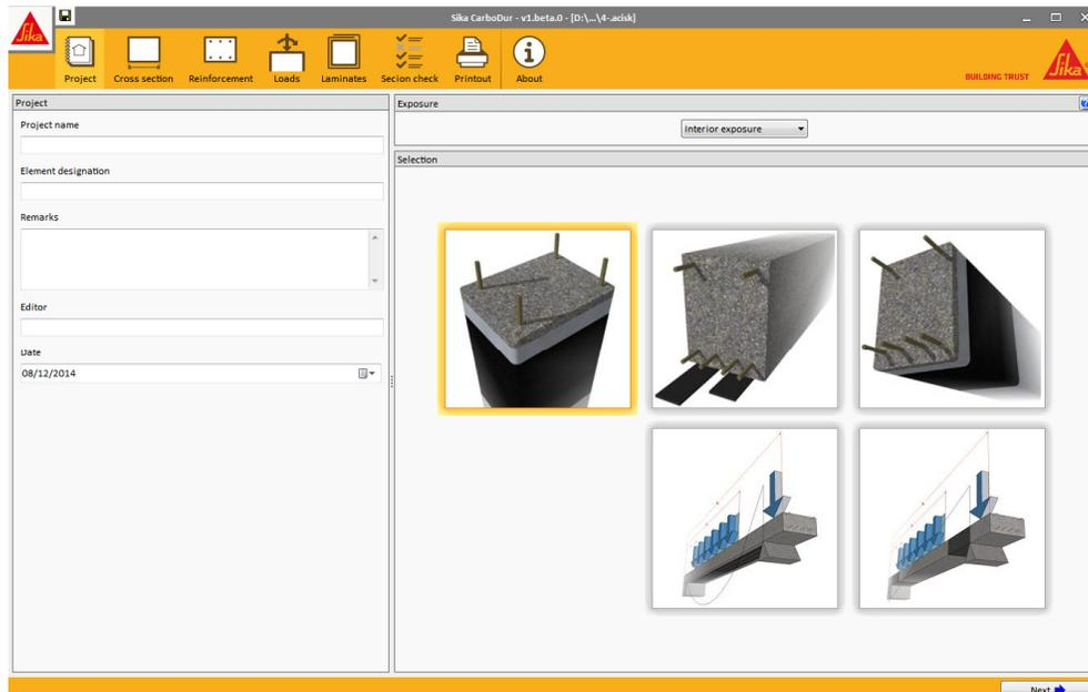
The selection of the type of strengthening is done by selecting one of the main drawings shown in the main screen:
