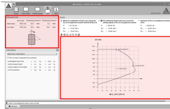
In case of a combination of axial load and bending moments, the software will display a 2D P-M interaction diagram showing the limit boundaries for the different situations as exposed below.
