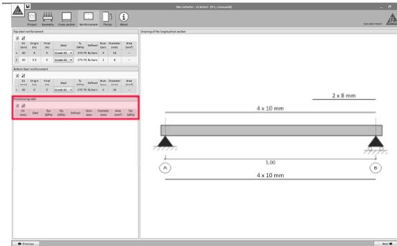
For elements based on simple supported beams comprising a single span, the use of prestressed steel is allowed by the software. The user must indicate the effective stress level in the prestressing steel, which corresponds to the original prestressing stress minus the corresponding stress relaxation at the moment of strengthening.
