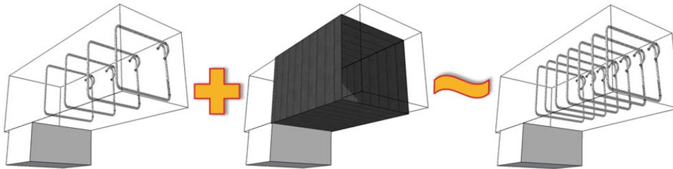
The effective strain depends on the degree of CFRP debonding when the shear capacity of the RC is reached; on in other words, on the type of anchorage (properly anchored CFRP, e.g. closed jackets, versus poorly anchored FRP, i.e. open jackets).
