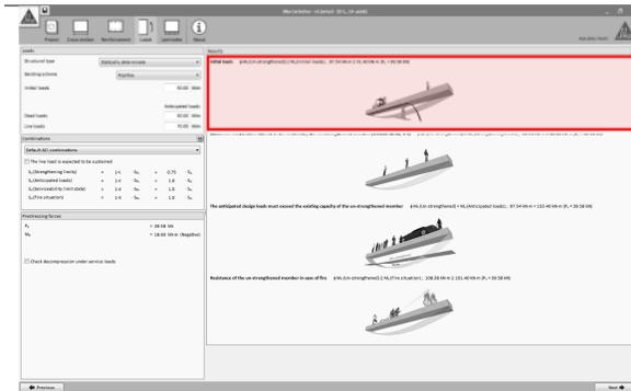
The main screen displays the preliminary checks concerning the performance of the unstrengthened member when compared to the anticipated loads entered by the user.
