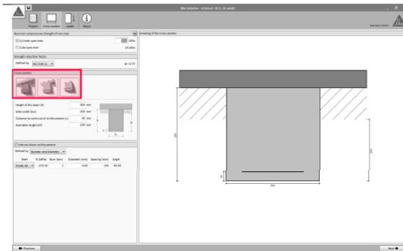
The drawings on the left area are used to select the cross-section of the member.
