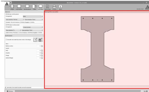
Finally, the main screen will show the necessary FRP arrangement as per the results of calculation.
