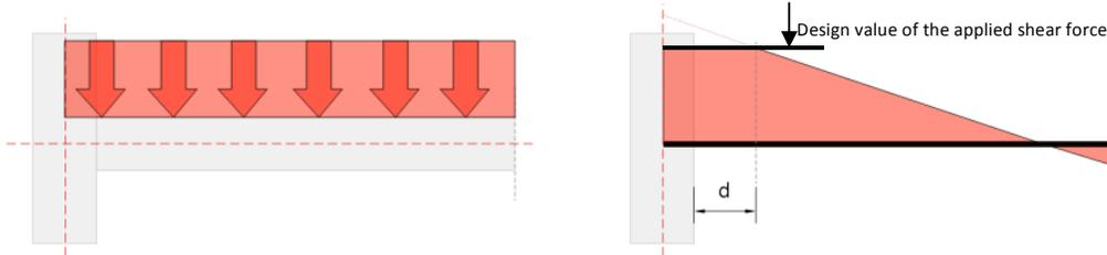
The external FRP reinforcement may be treated in analogy to the internal steel (accepting that the CFRP carries only normal stresses in the principal CFRP material direction), assuming that at the ultimate limit state in shear (concrete diagonal tension) the CFRP develops an effective strain in the principal material direction,  $\epsilon_{fe}$ , which is in general, less than the tensile failure strain,  $\epsilon_{fu}$ .
