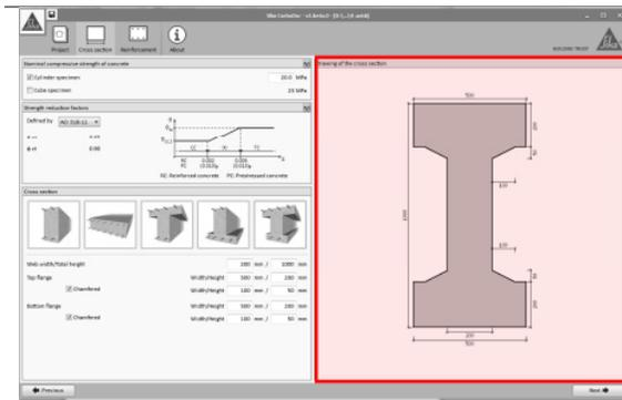
The final section and its dimensions are shown on the main screen.
