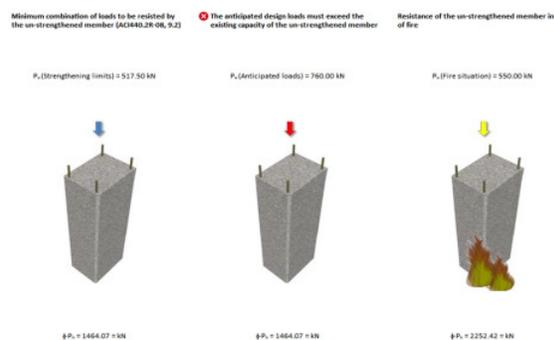
The first drawing (left) verifies if the existing member is able to support a reduced combination of the loads (top) entered by the user. The admissible load level is indicated at the bottom. This condition must be fulfilled to continue with the calculation.
