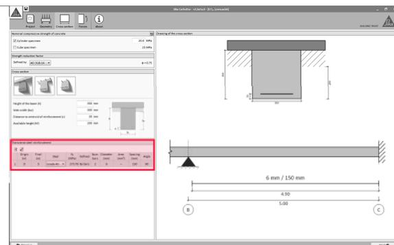
The transverse steel reinforcement must be defined for the whole span. Due to this, the user can enter different steel configurations (spacing, diameter, angle, steel grade...) for different segments of the span.
