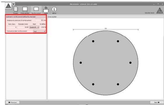
In case of circular columns, the vertical bars are distributed homogeneously around the perimeter.
