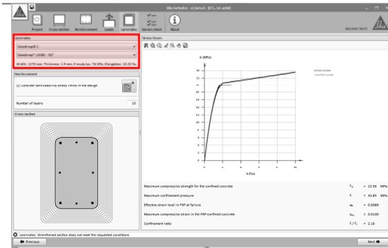
The selection of the Sika® product range is done by means of the drop boxes displayed on the upper left corner. Additionally, some simplified information concerning the selected system is shown immediately below.
