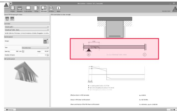
The software determines the necessary arrangement of the FRP laminates according to the expected loads and the strength of the original element.
