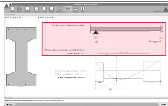
The software determines the necessary arrangement of the FRP laminates according to ACI 440.2R-08, 13.1.
