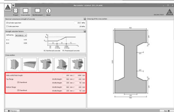
The main dimensions of the section are entered in the boxes shown beneath the schemes. Additionally, chamfers can be displayed for certain shapes, providing the possibility of defining complex geometries.
