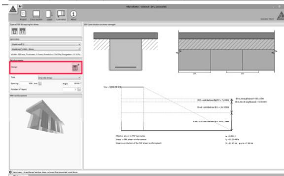
The automatic calculation of the FRP (calculator icon) will take into account the selected wrapping scheme, the type of FRP laminate and strips configuration (discrete strips or full wrapping).
