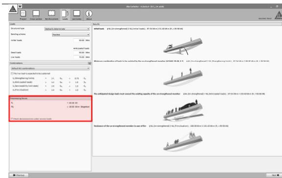
In case of prestressed members, the force and moment as resulting of the prestressing will be shown below the ACI combinations. For statically indeterminate members, the effective values must be manually entered by the user.
