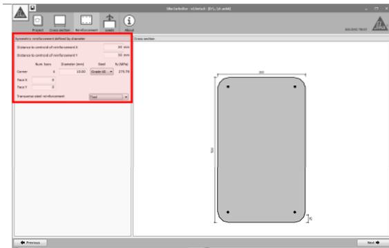
For rectangular sections, the reinforcement is defined by the steel located in the corners. Additionally, intermediate steel bars can be displayed along the horizontal and vertical sides of the section.
