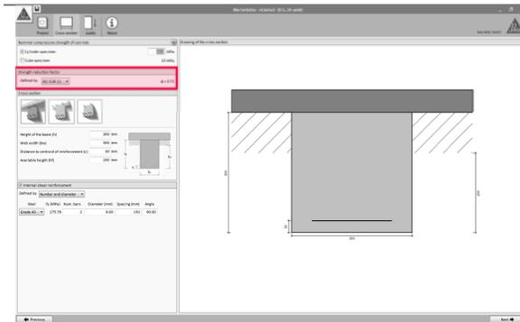
The design strength provided by a member shall be taken as the nominal strength of the member in accordance to ACI 318 and ACI 440.2R-08, multiplied by the strength reduction factor  $\phi$ .
