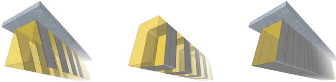
Closed jackets or properly anchored strips are always preferable compared with open jackets, as in the latter case CFRP premature debonding is usually expected; hence the effectiveness of the CFRP is reduced. 2-sided configuration provides the least effective performance due to the risk of debonding.
