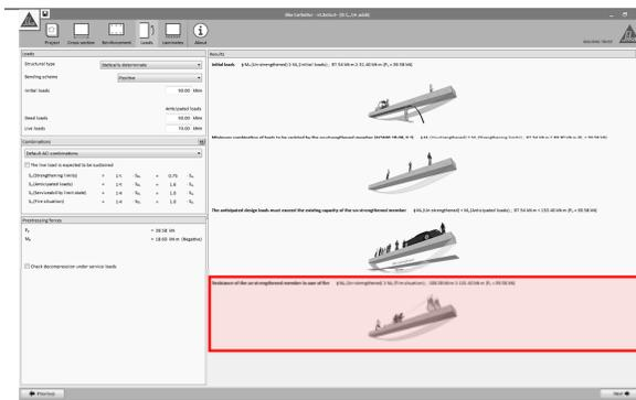
The last picture shows if the acting load in case of fire can be initially assumed by the unreinforced element (considering that the unprotected FRP is damaged due to the high temperatures). Otherwise the software will allow the calculation, but the printout document will remind the need of protection for the FRP.
