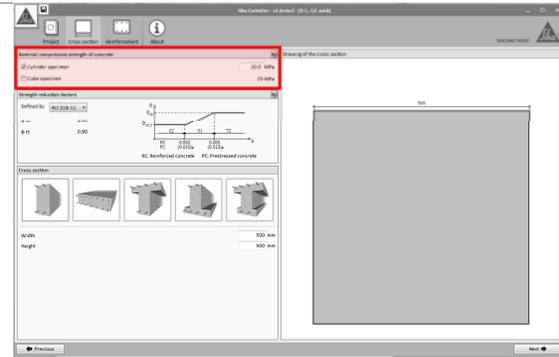
The compressive strength of the concrete ( $f'_c$ ) must be defined by the user.
