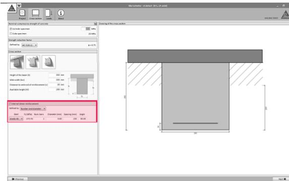
The internal shear reinforcement can be defined as a cross section or according to the distribution and geometry of the bars.
