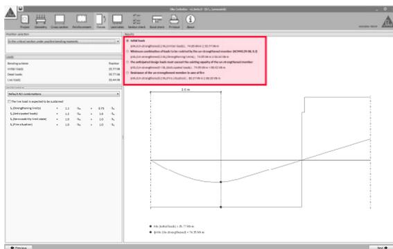
The main screen displays the preliminary checks concerning the performance of the unstrengthened member when compared to the anticipated loads entered by the user. The user can toggle the diagram shown in the main screen by clicking the corresponding option.
