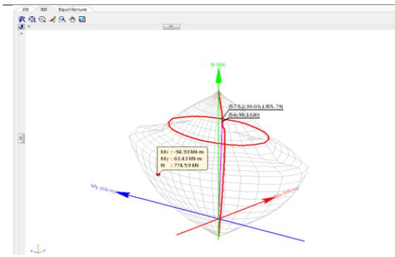
The 3D option displays the ultimate strength of the strengthened member, as well as the position corresponding to the combination of design loads. The user can obtain information regarding different combinations of moments and axial loads by positioning the pointer in any of the vertex of the grid's surface. The 3D model can be rotated and zoomed, as well as exported to diverse graphic formats.
