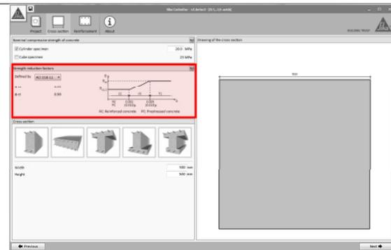
Design strength provided by a member shall be taken as the nominal strength of the member in accordance to ACI 318 and ACI 440.2R-08, multiplied by the strength reduction factor  $\phi$ .
