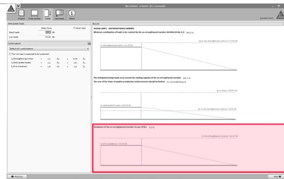
The last diagram shows whether the acting load in case of fire can be carried by the unreinforced element (considering that the unprotected FRP is damaged due to high temperatures). Otherwise, the software will allow the calculation, but the printout document will remind the use of the need of FRP protection.
