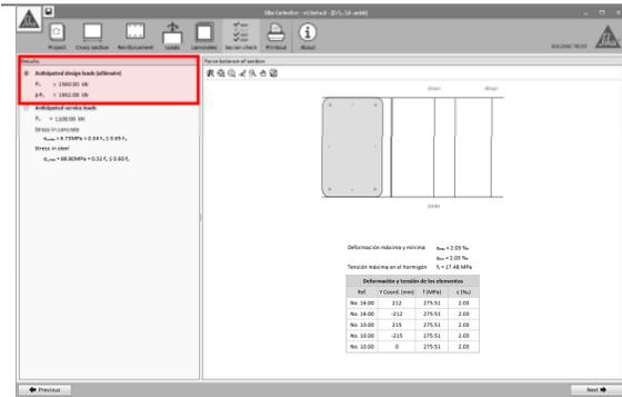
This section allows the user to know the resulting stress-strain states for the section under the combination of design (factored) loads or service loads.
