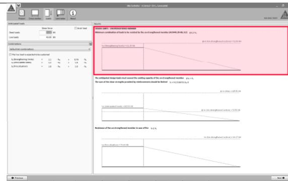
The first condition verifies if the existing member is able to support a reduced combination of the loads entered by the user (Refer to page 4 for additional information). This condition must be fulfilled in order to continue with the calculation
