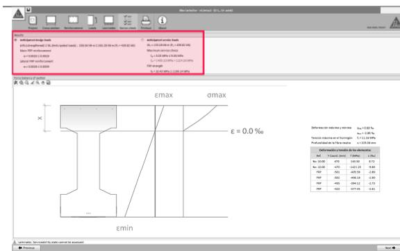
This section allows the user to know the resulting stress-strain states for the section under the combination of design (factored) loads or under service loads.
