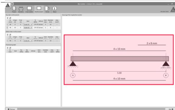
The main screen will display the steel arrangement as defined by the user.
