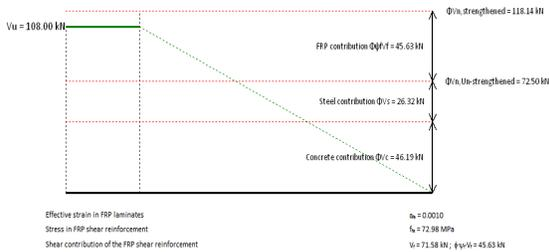
Finally, the FRP contribution to the strengthening will be displayed alongside the strengths corresponding to the existing steel reinforcement and concrete section.
