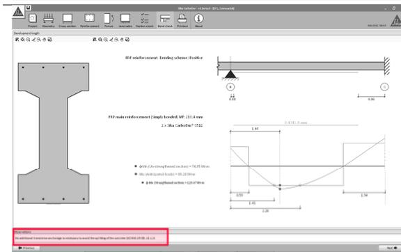
Verification concerning the end peeling of the FRP (ACI 440.2R-08), is displayed at the bottom. In case that the factored shear force at the termination point is greater than  $\frac{2}{3}$  the concrete shear strength, the FRP must be anchored to prevent the concrete cover layer from splitting.
