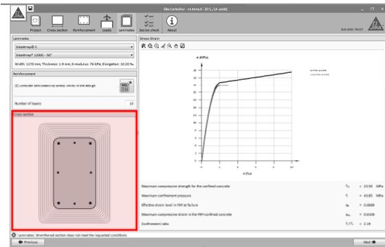
A schematic drawing on the left shows the necessary number of SikaWrap® fabrics.
