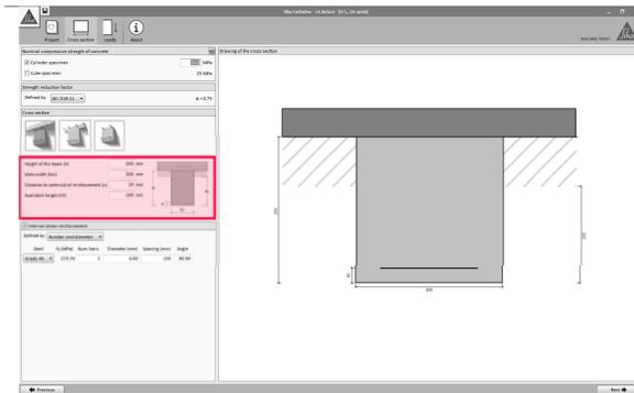
The main geometry of the beam is defined by means of the text boxes on the left. Note that the available height for the FRP may be restricted as a consequence of the existence of mortars or panels beneath the slab or the flanges.
