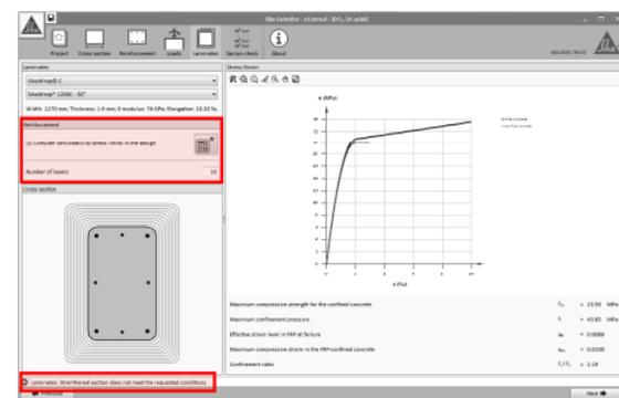
The calculation is done when the Calculator icon is clicked, showing the necessary number of plies corresponding to the selected SikaWrap® laminate.
