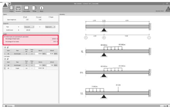
The initial, un-factored loads acting during strengthening must also be defined.
