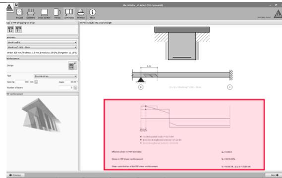
The shear diagram on the main screen displays the bending moment distribution corresponding to the anticipated design loads, as well as the original strength of the un-strengthened member.
