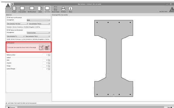
The dimensioning of the FRP reinforcement can take into account the Serviceability stress limits by enabling the corresponding option (otherwise it will be based only on the Ultimate Limit State of the member).
