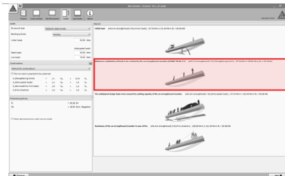
The second condition verifies if the existing member is able to support a reduced combination of the loads entered by the user (Refer to page 4 for additional information). This condition must be fulfilled to continue with the calculation
