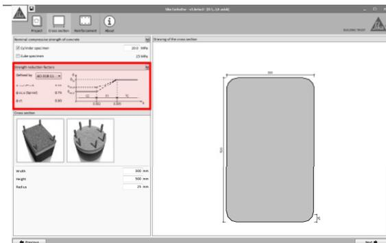
Design strength provided by a member shall be taken as the nominal strength in accordance to ACI 318 and ACI 440.2R-08, multiplied by the strength reduction factor  $\phi$ .
