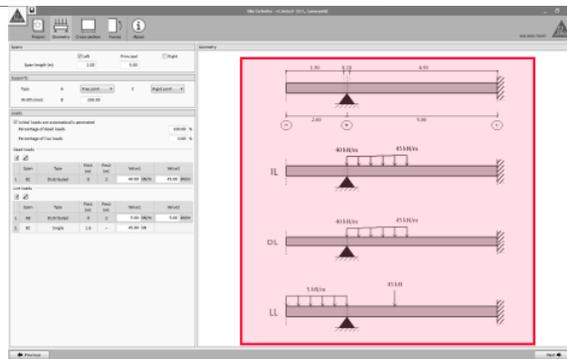
The schemes in the main screen display the arrangement of the loading as defined by the user, and are divided into:
