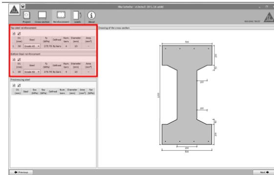
The definition of the top and bottom steel bars is done individually for each layer, comprising the following parameters:
