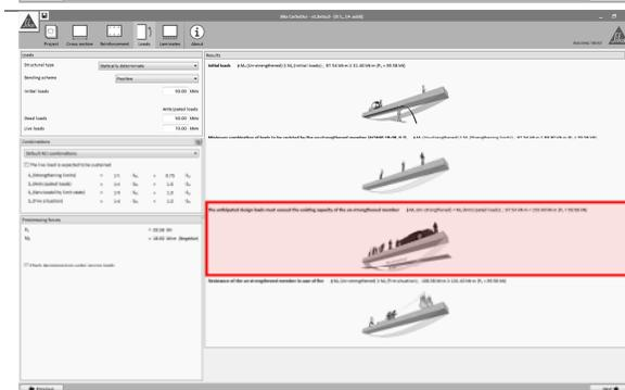
The 3<sup>rd</sup> scheme checks that the requested loads exceed the strength of the existing, unreinforced member. This condition must be obviously verified to continue with the calculation.
