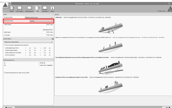
CFRP strengthening is feasible either for negative bending moment or positive bending moment. The kind of calculation must be chosen in the corresponding dropdown box.
