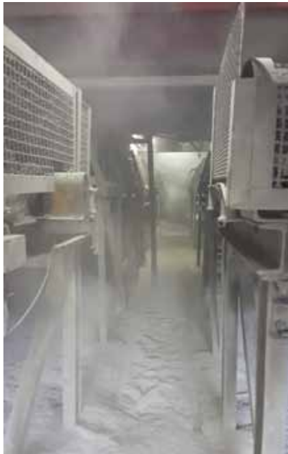
Figure 3: dust formation in the mill house due to the high dispersion power of grinding aids
