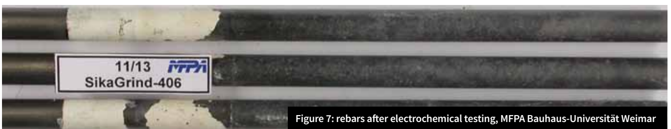
Figure 6: electrochemical test according to EN 480-14:2007-03, MFPA Bauhaus-Universität Weimar
