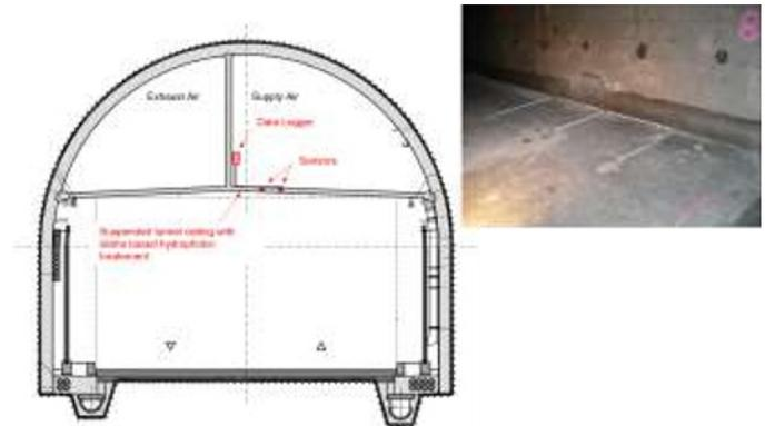
Figure 1. Schematic / photograph of the installed monitoring system in the tunnel.
