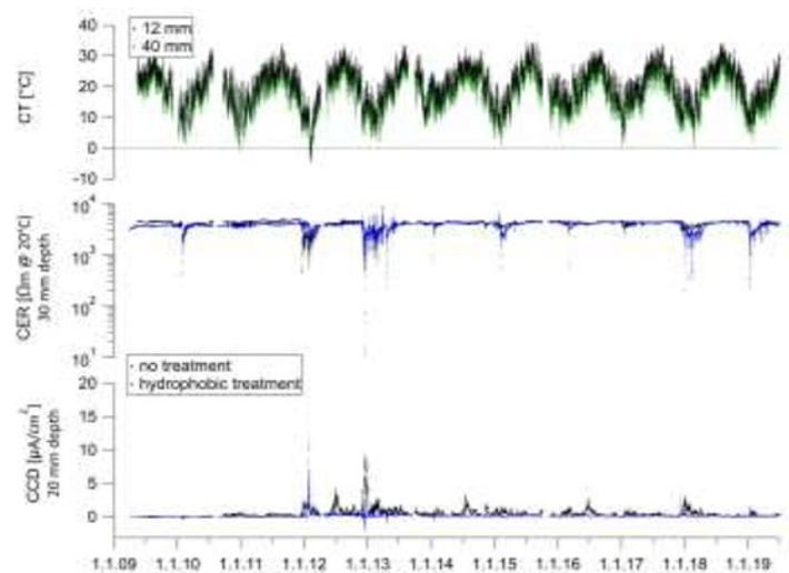
Figure 5. Temperature change at different depths, CER and CCD for untreated (black) and treated (blue) concrete during a 12-year period, 287 m from the tunnel north portal.
