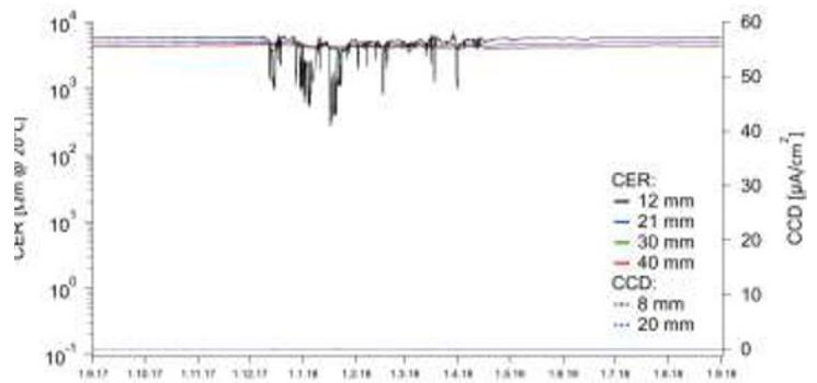
Figure 4. The CER and CCD of a silane treated concrete during a reference year 240 m from the tunnel portal.
