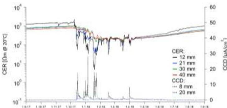
Figure 3. The CER and CCD of an untreated concrete during a reference year 240 m from the tunnel portal.
