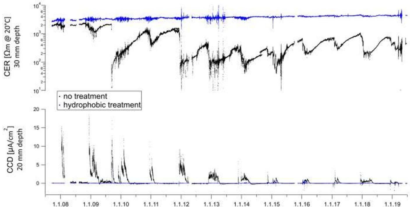
Figure 2. CER (top) and CCD (bottom) of an untreated (black) and a treated (blue) concrete 240 m from the tunnel south portal during a 12-year period.
