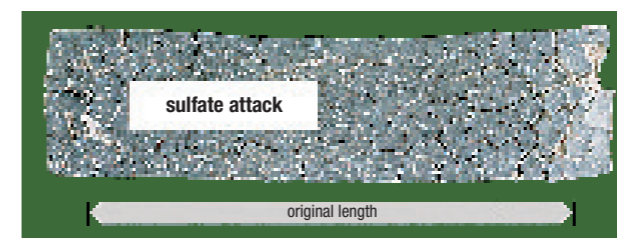
Sulfate driven attack is primarily caused by sulfates dissolved in water. By reacting with the hardened cement matrix, an increase in volume is induced, which damages the structure. (Picture: BetonSuisse, Merkblatt 01)
