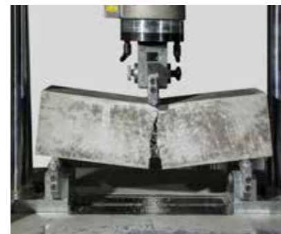
Beam test: EN 14651
