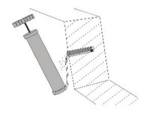
2. Thoroughly clean the drill hole with a steel brush. Note: The diameter of the brush must be larger than the diameter of the drill hole. Clean the drill hole a minimum of two times.
