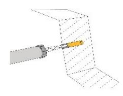
3. IMPORTANT Place the anchor within the open time. Insert the anchor with a rotary motion into the filled drill hole.
