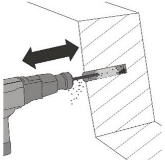
IMPORTANT Use oil-free compressors. Start from the bottom and clean the drill hole using an air lance, pressure: 6 bar (90 psi).
