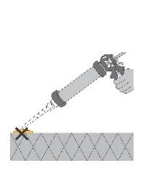
2. IMPORTANT Do not entrap air into the drill hole. Inject the Product into the drill hole starting from the bottom, while slowly drawing back the static mixer. Note: For deep drill holes, extension tubing can be used.
