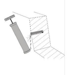
CLEANING DRILL HOLES WITH DIAMETER DO > 2 20 MM AND EMDEDDED DEPTH > 240 MM
