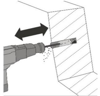
3. IMPORTANT Use oil-free compressors. Clean the drill hole with a blow pump or by compressed air, starting from the bottom of the drill hole.
