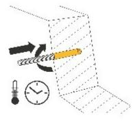
4. Do not load or move the anchor during the hardening time.
