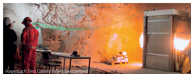
In special furnace chambers fire trajectories can be replicated, panels tested and subsequently evaluated. Temperature development is measured at various depths and recorded.
