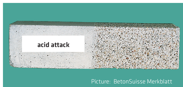
Acidic solvent attacks which dissolve calcium compounds out of the hardened cement matrix can be caused by acids, exchangeable salts, vegetable or animal fats or oils. Degradation of the concrete usually occurs very slowly.
