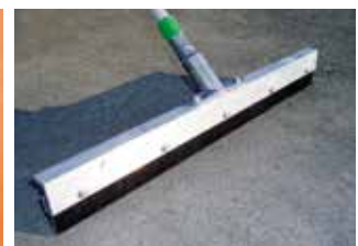
Sealing of broadcast layers with a straight trowel or a "squeegee" blade.
