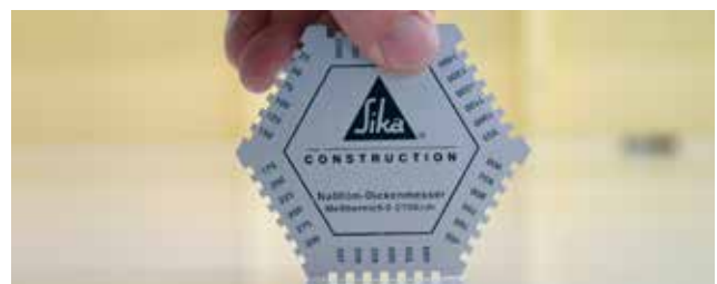
Wet Film Thickness gauge for coatings application thickness control.
