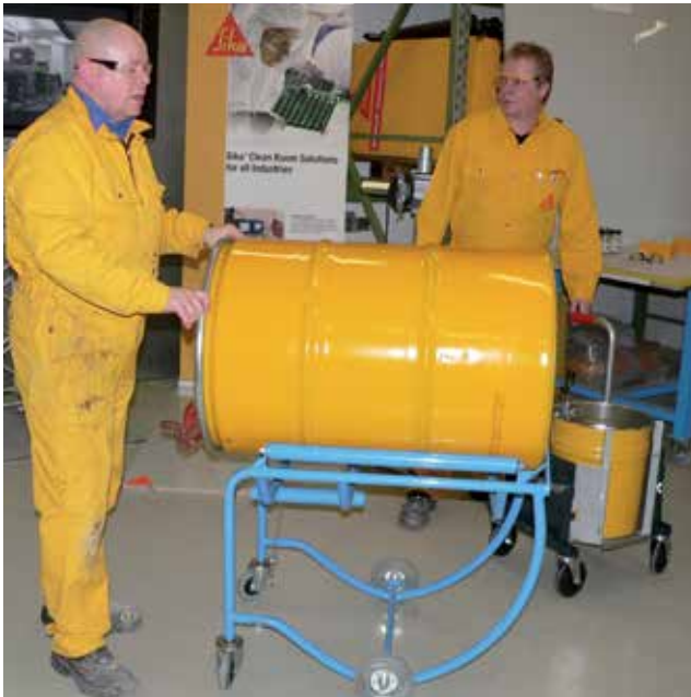
Barrel-cart: modified for drum handling with the Application Trolley.
