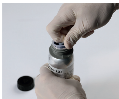
Fig. 23 Close inner cap immediately after use
