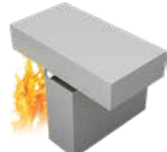
12. Single seal, exposed side
