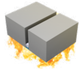
9. Single seal, exposed side
