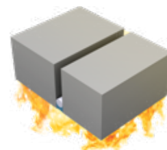
9. Single seal, exposed side
