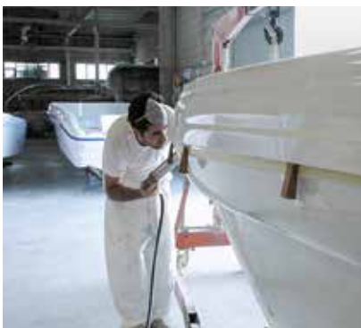
Fig. 8 Sealing with Sikaflex®-295 UV
