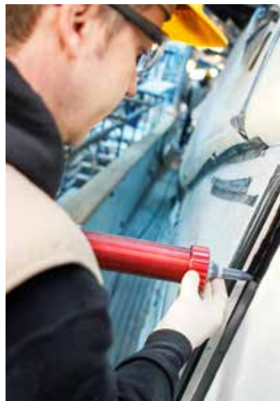
Fig. 6 Adhesive is applied to the window frame
