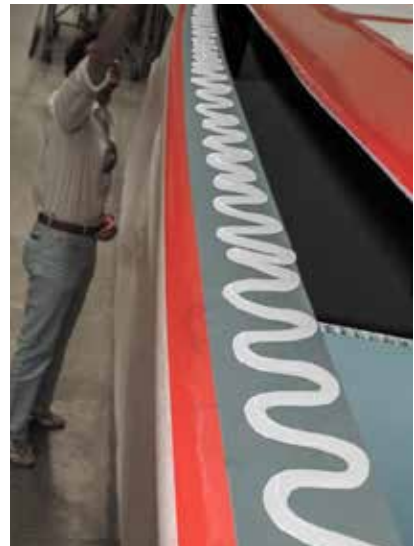
Fig. 9 Hull and deck are brought together
