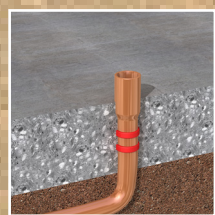
Sealing of penetrations
